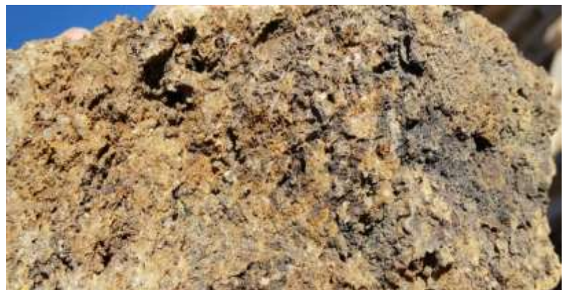
Figure 3 - Gold mineralization (2.55g/t Au) in basement granite with vuggy silica alteration (DDH-07-32 240m)
